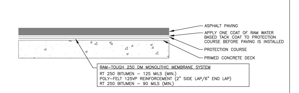
NOTE: BEFORE PAVING, USE BARRETT HYWAY TACK COAT, DO NOT USE SOLVENT BASED TACK COAT.
